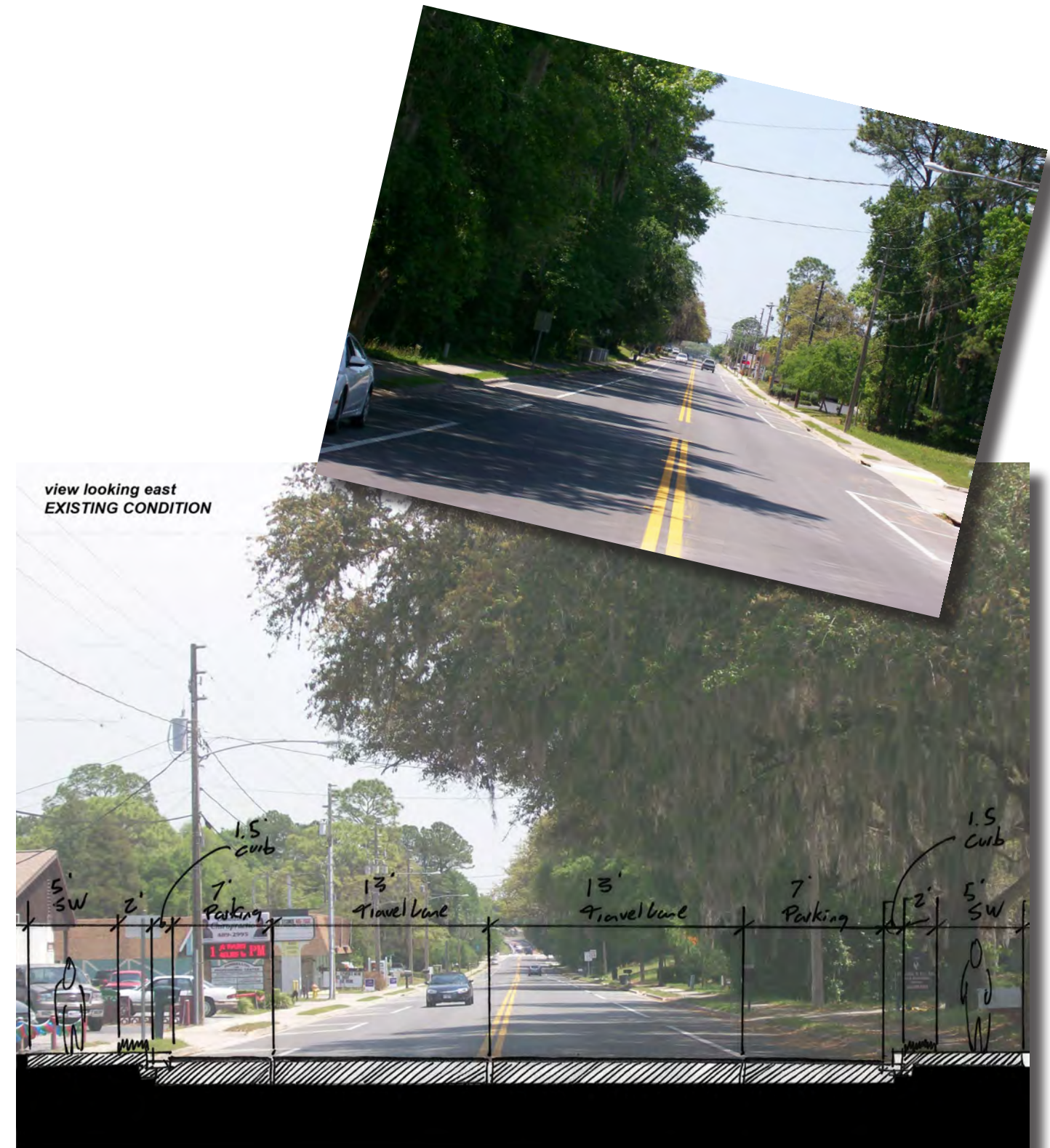
Existing Pennsylvania Avenue typical section
