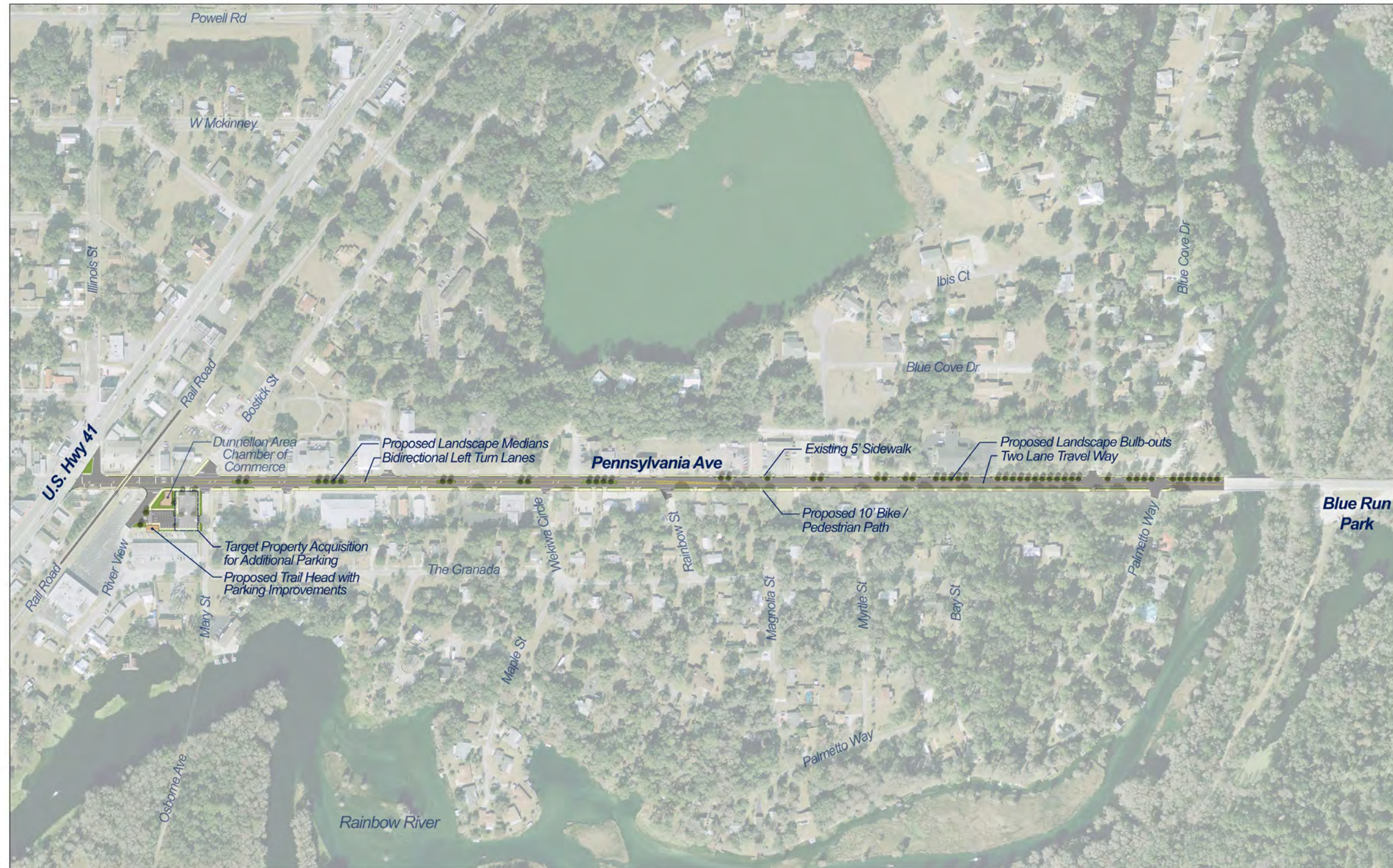
Figure 9A: Pennsylvania Avenue Streetscape Plan View
